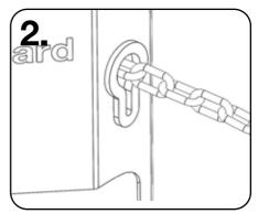
Slacken the chains by lifting them up from the slot in the hawsehole and pulling through from the front to the transformer.
