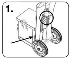
Butt the rubber pads against the transformer and unclip the hooks from the holes on the back of the T-Kart.
