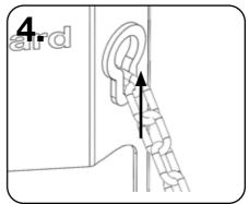
Tighten the chains again by lifting the chain link in the hawsehole and pull through from the back of the T-Kart. Then lock in the position as shown.
