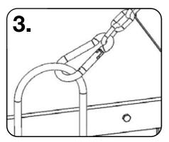
Use the clip hooks to attach both chains to the hoops/handles of the transformer.
