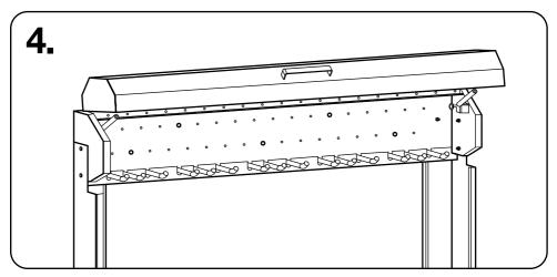
Using at least 2 people, stand the unit up into position, preferably with its back to the wall. For added security, using the pre-drilled holes in the head unit, bolt the StrimmerSafe Rack to the wall before loading.
