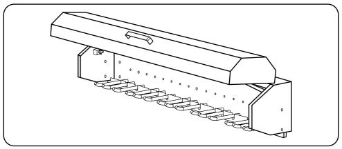
The head unit can be fitted to a wall without the base unit and side sections. Using the pre-drilled holes in the back of the head unit bolt back to the wall. Ensure the unit is securely fixed to the wall before use.
