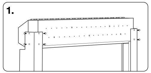
Position the head unit on the floor face down. Bolt on the side panels to the head unit using 4 of the M8 x 20 bolts and Nylocks on each of the upright arms.
