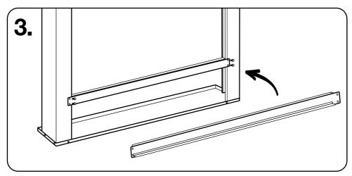
Attach the cross brace using 2 of the M8 x 20 bolts and Nylocks each side. Ensure all fixings are secure and tight.
