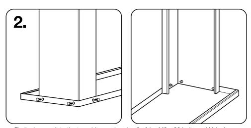
Fix the base unit to the two side panels using 3 of the M8  $\times$  20 bolts and Nylocks on each of the upright arms.
