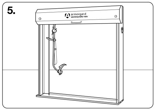
Open the lid of the StrimmerSafe Rack and position the head of your tools over the internal hooks. Close the lid of your StrimmerSafe Rack and secure both locks Your tools are secure with the Armorgard StrimmerSafe Rack.
