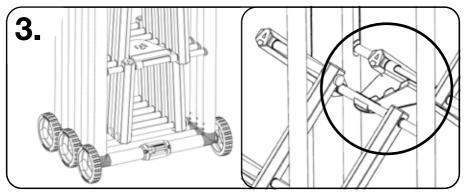
Built in latch locks the InstaGate in the retracted position, or can be used to daisy chain other InstaGates together.
