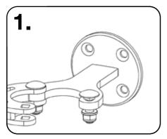
The anchor kits are sold individually, to enable the InstaGates to be secured to a surface.
