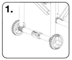
All InstaGates have four braked wheels to enable it to be locked in place.
