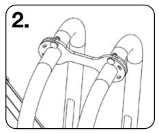
The ideal position when connecting InstaGates in a straight line is a link on both the top and the bottom horizontal bars of the InstaGates.
