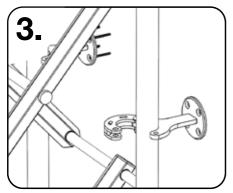
Simply push your InstaGate into the anchor, and swing the end around to align the bolt holes.
