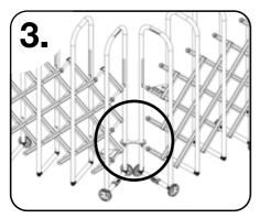
If connecting InstaGates on an angle, or connecting different size InstaGates, place the linking kit on the uprights.
