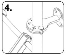
Use the included M8 bolt and nylocks to fasten the anchor kit in place. For more efficient use, a padlock can be used instead as shown in step 4 on page 9.
