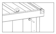
**5.** Feed the loose end of cable from the lighting kit through the hole and clamp it tightly using the gland.
