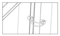
**5.** Fix pipe linchpins in each corner, and bolt in the 20mm bolts to secure it to the base.
