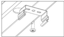
2. Using a 5.5 self-drilling screw, attach the light bracket to the roof using the pre-drilled holes. Repeat these steps to install the second bracket.
