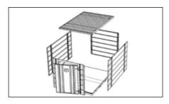
To dismantle the Forma-Stor, remove the parts in reverse order to which they were assembled.
