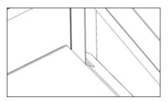
Rest the shelf into position. It will need to align with the corner of the unit with one of its cut-outs. Repeat the steps to install the other shelves.
