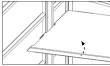
2. Locate the relevant inner slots on the back panel, and position the shelf by tilting and inserting the pocket on its edge into the back vertical support of the side panel.
