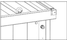
4 Locate the 20mm hole located in the top corner of the Forma-Stor's side panel, and fit the compression gland into the hole by screwing it tight.
