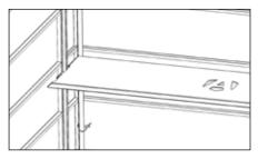
Each size Forma-Stor unit can fit up to five shelves. Do not exceed the 200kg UDL the shelf was designed for. No fixings are required for shelves.
