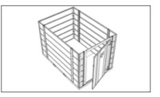
The door panel is the last panel to be fixed on. This slots onto the base and is fixed to the side panels with linchpins and bolts as described in step 5. It is easier to do this with an extra person inside.
