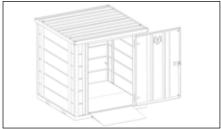
When using the ramp, do not exceed the 1 tonne UDL that it was designed for. Do not close the door whilst the ramp is in position.
