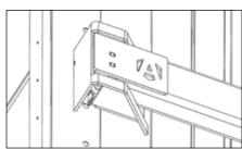
Remove the bar by pulling it and sliding it to the left. This will allow the access to the door's locking system.
