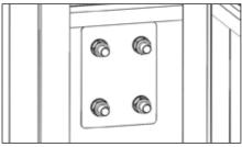
Inside the Forma-Stor, replace with the blanking plate and then place a washer and nylock nut on each bolt. Repeat for both housings.
