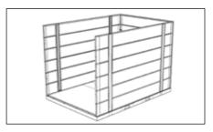
Place the other side panel on the base, and secure it with bolts and linchpins as described in steps 3 to 5
