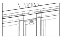
**11** Lastly, fix the roof in place using the 45mm bolts provided. Tighten all the bolts in the Forma-Stor.
