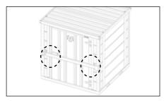
To install the BlokkaBar, locate the pre-drilled holes on either side of the door. Then, remove the coach bolts and blanking plate.
