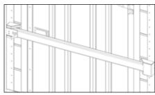
Place the lock housing of the BlokkaBar on the left side of the door. The other housing should be placed on the right side of the door.
