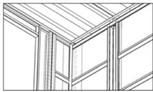
**10.** Ensure the grooves in the roof fit securely to the top of each of the four panels.
