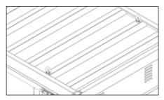
Before lifting, ensure that the bolts holding the lifting eyes are securely in place.
