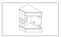
**3.** Ensure the padlock is located in the locking housing with the lock facing down. Push the coach bolts through the holes in each housing and place into the pre-drilled holes in the Forma-Stor.
