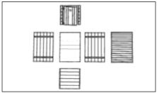
Remove the roof first, followed by the door panel, a side panel, the rear panel, and then the remaining side panel. Fixings can be bolted back into the panels for safekeeping.
