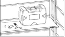
Test the shelves by pushing down with force and ensuring it doesn't slip before loading with any contents.
