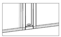
**3.** Ensure it is supported safely whilst you use the 45mm bolts to secure the side to the base. Leave all fixings loose at this point.
