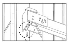
To unlock the BlokkaBar, place the key in the keyhole of the lock on the bottom, and turn. This will unlock, releasing the pin.
