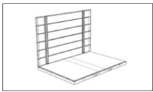
Place one of the side panels on the base, and use the 20mm bolts at each end to locate the panel.
