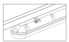
Check that brackets are secure, and then clip the light into the brackets.
