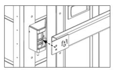
To lock for maximum security, ensure that the Forma-Stor door is locked before placing the BlokkaBar. Slide the bar in place.
