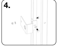
Fit the mounting brackets for the folding bench to the inside of each rear upright using 2x M8x25mm bolts, washers and Nylocks per side. Use a 13mm spanner/socket to ensure these fixings are tight.
