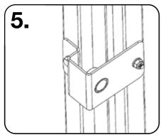
Slot the lugs of the folding bench into the brackets and tighten rear uprights to base.
