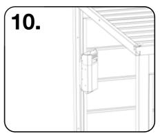
The cigarette bin can slot into any upright without fixings. To remove, lift upwards and out.
