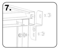
Next the middle supports for side panels need to be fitted, one on the back and each side. Slide the top of the support under the roof first and then fix to the base using M12x25mm bolts and washers. The top can then be fixed using the supplied bracket and M12 fixings as shown.
