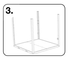
Tighten the two front uprights using a 19mm socket but leave the rear uprights hand tight.
