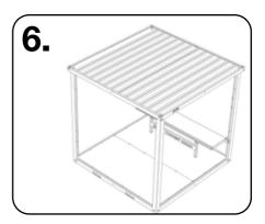
The roof can now be lifted onto the uprights and located by the channels running under the roof in each corner.
