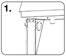
At the rear of the CuttingStation is a blanking plate that can be removed to allow cables, extraction hoses etc to be fed into the cabinet beneath the work surface
