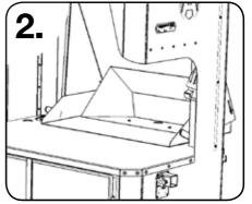
To extend or retract the panel, lift the handle on either side of the swarf collector and push or pull in the direction required.
