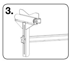
The support arm head can be turned 90 degrees for a v-shaped support to hold round materials. Note that in this position the flat surface can also be used as a stop for efficient cutting.
