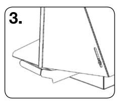
When the back panel is extended, the handles on either side drop down to lock it in position.
