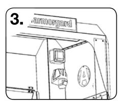
Inside the CuttingStation a switch is located in the top right corner for operating the work light.
