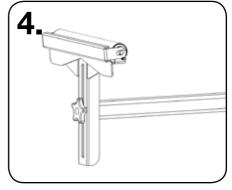
The last configuration is a roller, to enable materials to be repositioned easily while being supported at the same time.
