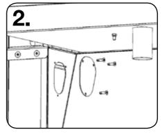
The plate can be removed and refixed with the three screws.
