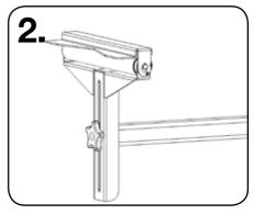
The support arm can be configured to have a flat support rest. We do not recommend extending the arms further than 800mm from the main unit.
