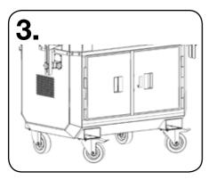
We recommend you position the two swivel-braked castors so they are at the front of the unit, and the two swivel castors at the rear.
