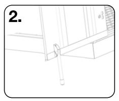
Door stays on the doors provide an easy way to safely and securely prop the doors open. Door stays must be disengaged before trying to close the door.
