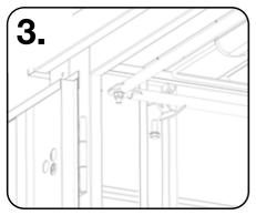
If curtain rails need to be removed then they should be unbolted carefully using the brackets.
