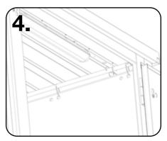
The sound deadening curtains are affixed using cable ties onto the rails provided. When removed for cleaning, these can be replaced very simply using more cable ties.
