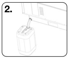
A sump plug is provided in the rear corner for easy disposal of slurry. The slurry must be collected into a suitable container such as a tank screwed onto the sump plug, and disposed of safely.
