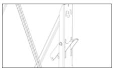
The Barricade has a latch that also functions as a carry handle when the Barricade is retracted and latched.
