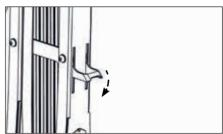
2 To latch or unlatch the Barricade, simply press the handle down, which then releases the catch.
