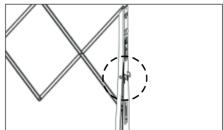
**2** To use the latch, fold the Barricade and fit the latch into the holes.
